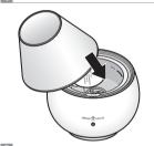
Make sure the retaining plate is correctly covering the vent ( as shown in the left diagram ) and the glass cover properly in place.
