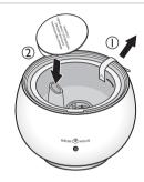
Remove the water level label and place the retaining plate into the vent in the tank. ( as shown in diagram left ) .
