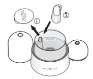
Remove the cover and lid first, then remove the retaining plate from the vent hole and replace it with the provided waterproof cap.
