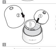
Make sure the retaining plate is correctly covering the vent ( as shown in the left diagram ) the cover and lid are properly in place. Use a clean cloth to gently wipe the surface of this Scentilizer, if needed.
